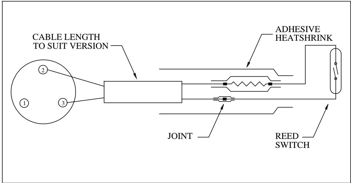
FIGURE 4 WIRING DIAGRAM OF ARG100/LX AND EC VERSIONS.
