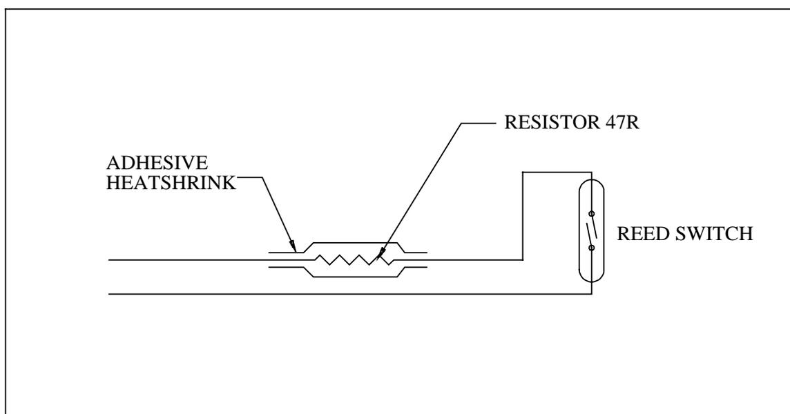
**FIGURE 3 WIRING DIAGRAM OF ARG100.**
