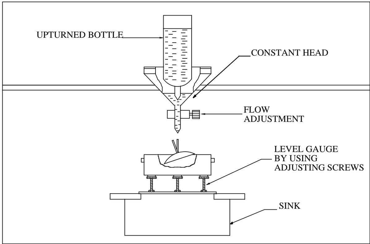
**FIGURE 6(b) DYNAMIC CALIBRATION (Constant Head)**
