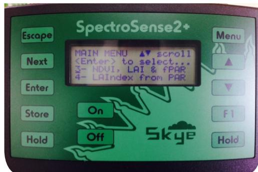
Logging display meter for visible/NIR light sensors
