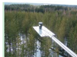
Skye 2-channel sensors on an Eddy-Covariance Tower. Courtesy: Dr. Caroline Nichol
