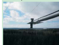
Skye 2-channel sensors on an Eddy-Covariance Tower. Courtesy: Dr. Caroline Nichol
