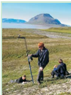
BSES expedition to Greenland. NDVI system used for the study of vegetation characteristics for low arctic vegetation
